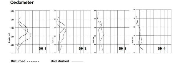
Figure 6 Oedometer Disturbed and Undisturbed Samples, June 2007
