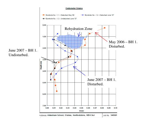
Figure 8 Enlarged Plot of Oedometer Results from BH 1
