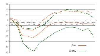
Figure 3 The precise level readings plotting ground movement from May 2006 through to June 2007.
